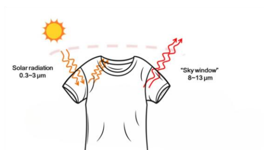
Figure 1: Schematic illustration for the mechanism of radiative cooling
