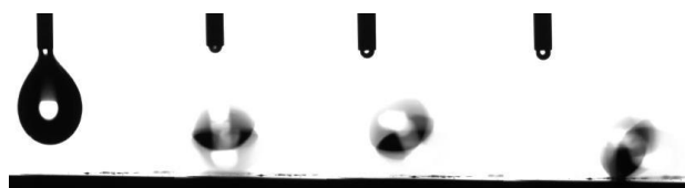
Figure 1. Water repellence of a stainless steel substrate coated with a nanohybrid film consisted of Protectosil WS 610 and SiO 2 nanoparticles following thermal annealing.
