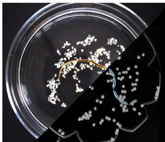
Figure 1. Collecting particles with active filamentous matter. (Top) A California blackworm ( Lumbriculus variegatus ) in a petri dish with sand particles. Over time, the worm gathers the sand into larger clusters. (Bottom) A robotic filament composed of connected “Hexbug” bots moves within a circular arena, interacting with passive (Styrofoam) particles. The robotic filament collects particles into clusters, mimicking the behavior of the living worm.
